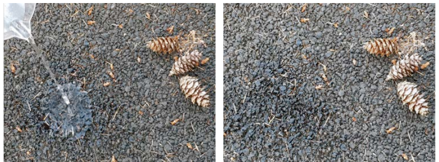
Water poured on permeable pavement quickly soaks in.
