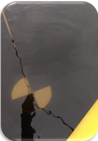
Secchi disc visible at 0.5 meters, disappearing at 1.2 meters (left); plankton net; green plankton (right)!
